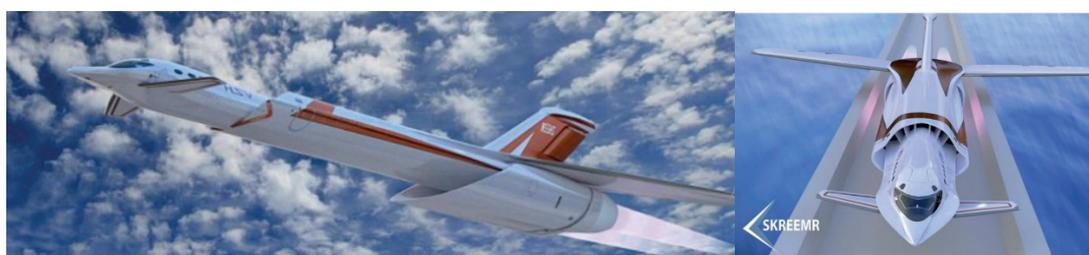
First off, to get the Skreemr jet to Mach 4, the aircraft is launched from a magnetic railgun launching system. This is a similar system to one that NASA is considering to help launch spacecraft, and involves a magnetic field accelerating the jet along a set of rails at incredible speed. It pretty much works in the same way as the maglev trains in Japan, which levitate the train carriage to avoid friction.
