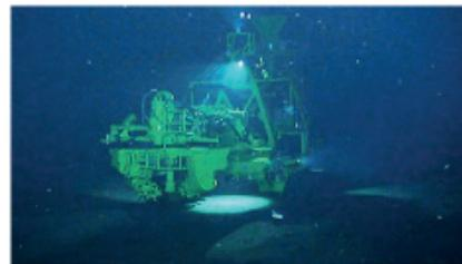
Ore-collecting test machine working on the seafloor
