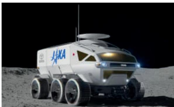
The six-wheeled rover will be powered by a **fuel cell** and be able to accommodate two people – or four in an emergency. Photograph: Toyota
