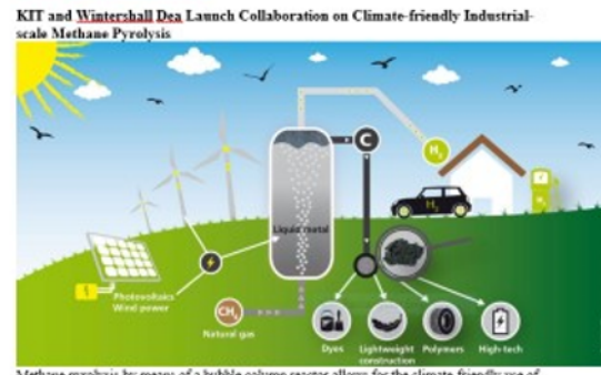
Methane pyrolysis by means of a bubble column reactor allows for the climate-friendly use of fossil natural gas. (Graphics: Leon Küster, KIT)
